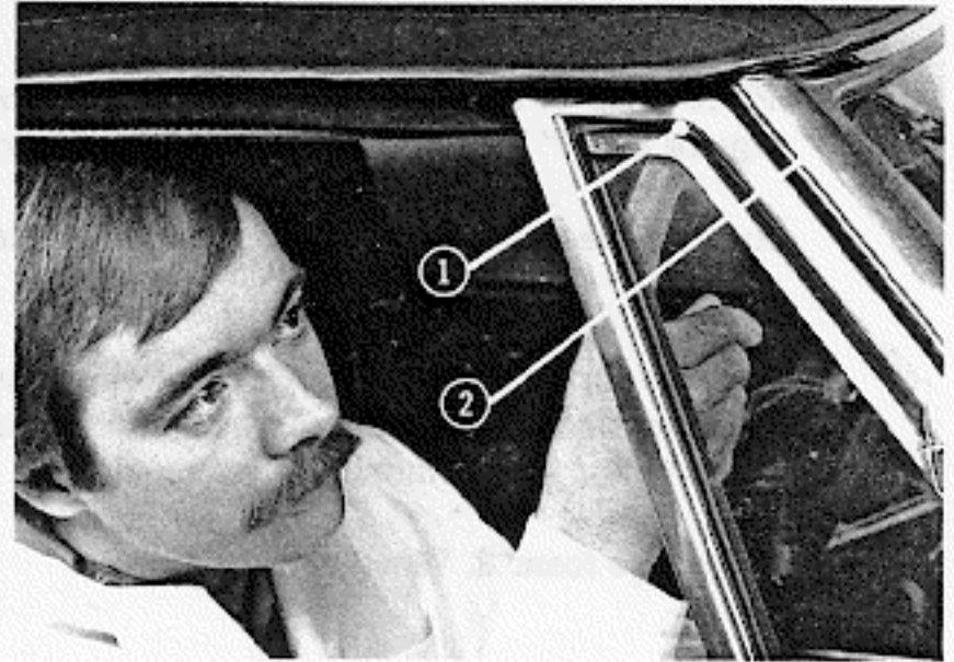
Checking vent frame seal.
