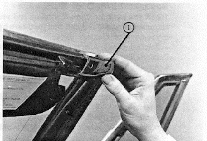
Removing corner molding.
